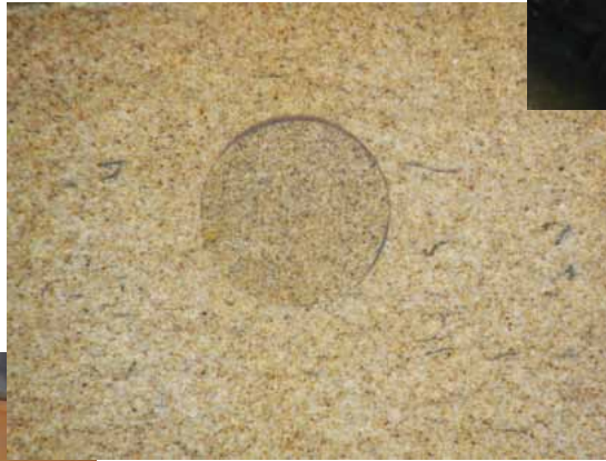
Figure 6. Circular indent installed with the use of two core bits. (Photo: Jasper Swann)
